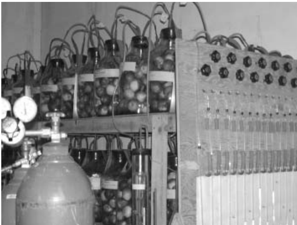
Figure 3. Experimental set up for treatment of fruit with 1%, 2.5% or 5% carbon dioxide (2% oxygen).
