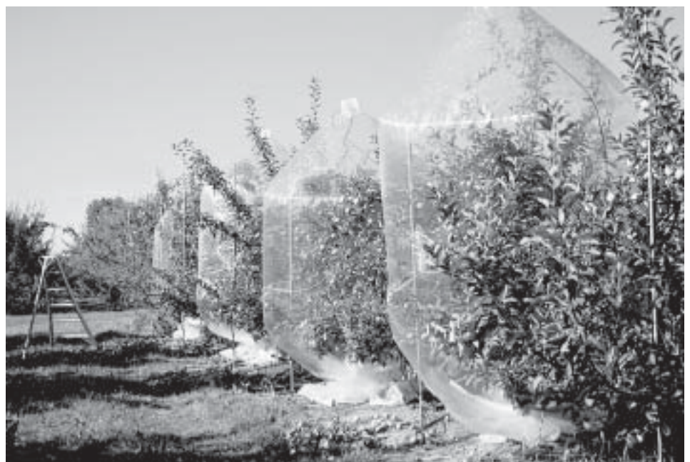
Photo 1. Clear "balloon" chambers used to control and monitor air flowing by apple trees help researchers measure the trees' photosynthesis and transpiration (water loss).
