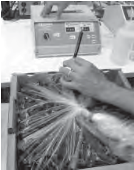
Figure 2. Gas measurements were taken weekly to determine the oxygen and carbon dioxide concentrations in the bags.
