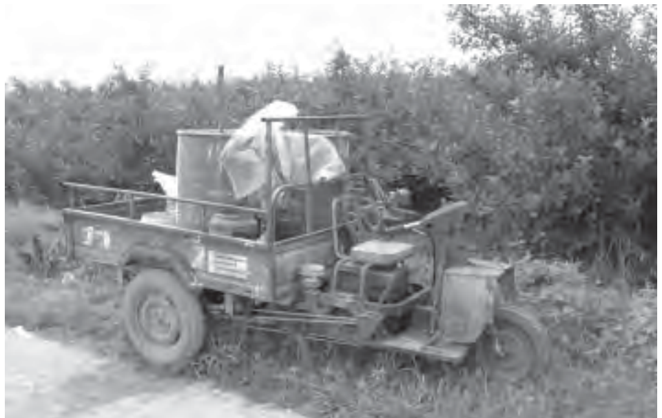
Figure 17. Three-wheeled hydraulic sprayer with 50 gallon tanks. Hoses were dragged into the orchard from access roads.
