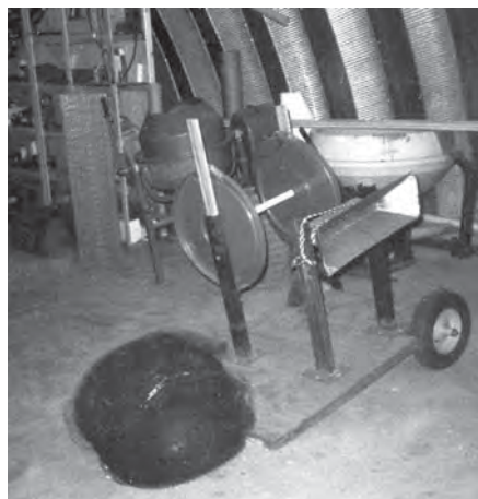
Figure 1. Derrick Farm homemade netting rewind machine with final roll (14'x300') beside it.
