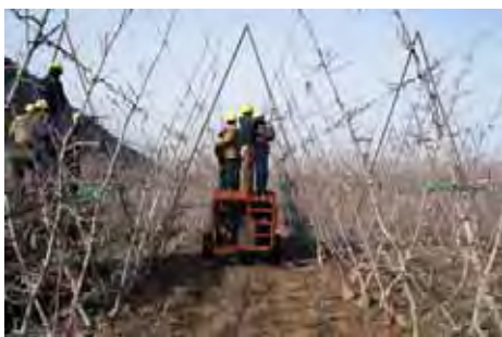
Figure 7. Self steering motorized platforms to improve dormant pruning efficiency.
